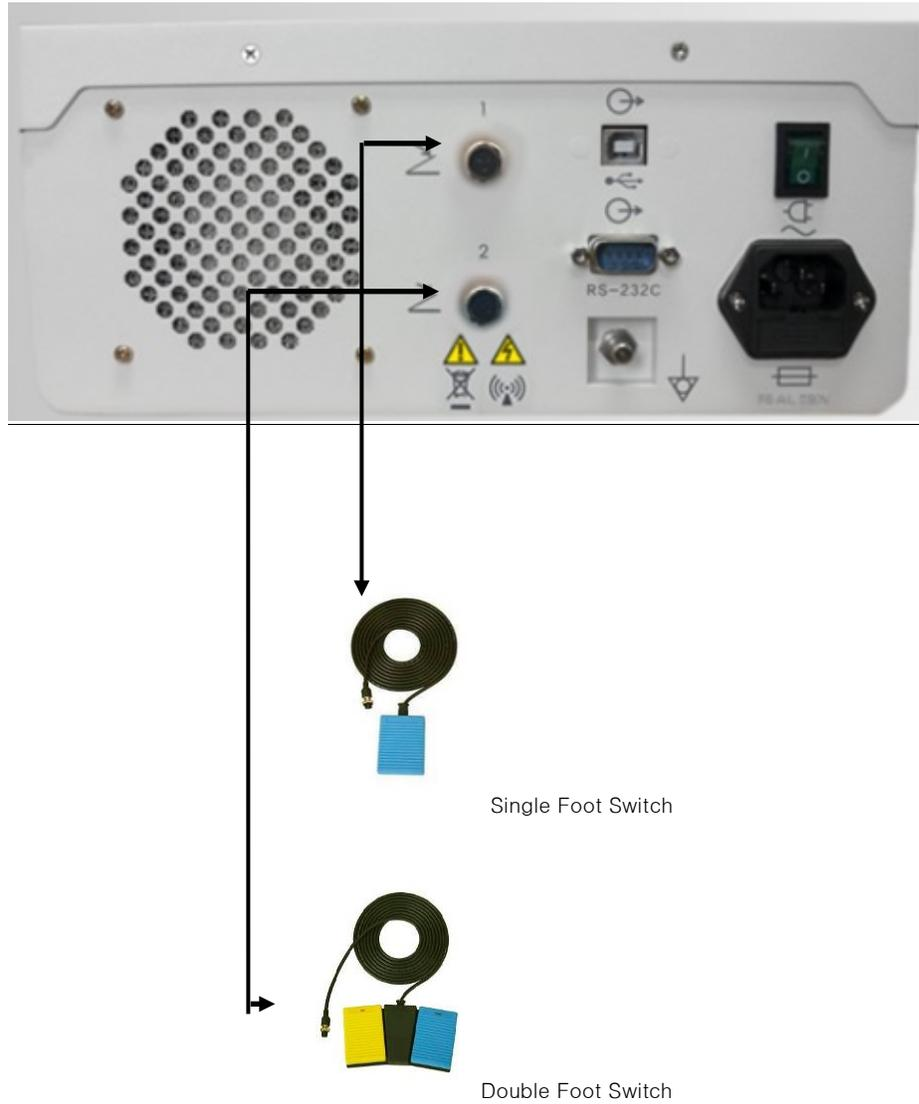
☞ Connect the foot switch. Then, tighten the screws.
